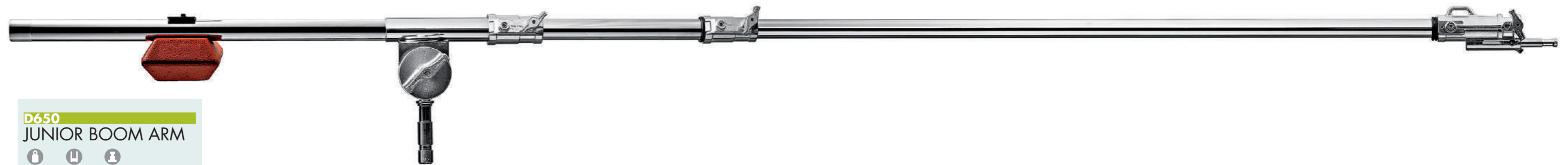
D600 MINI BOOM 3,6kg 16mm 7,9lb 5/8" Min extension 117cm (46.6"). Max load 30kg (66.1lb). Max extension 212cm (83.5"). Max load 7kg (15.4lb). 16mm (5/8") female stand attachment. D600CB MINI BOOM BLACK CHROME FINISH VERSION
