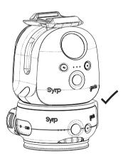
(!) IMPORTANT Ensure the Genie Quick Release base is fully inserted. It should be flush.
